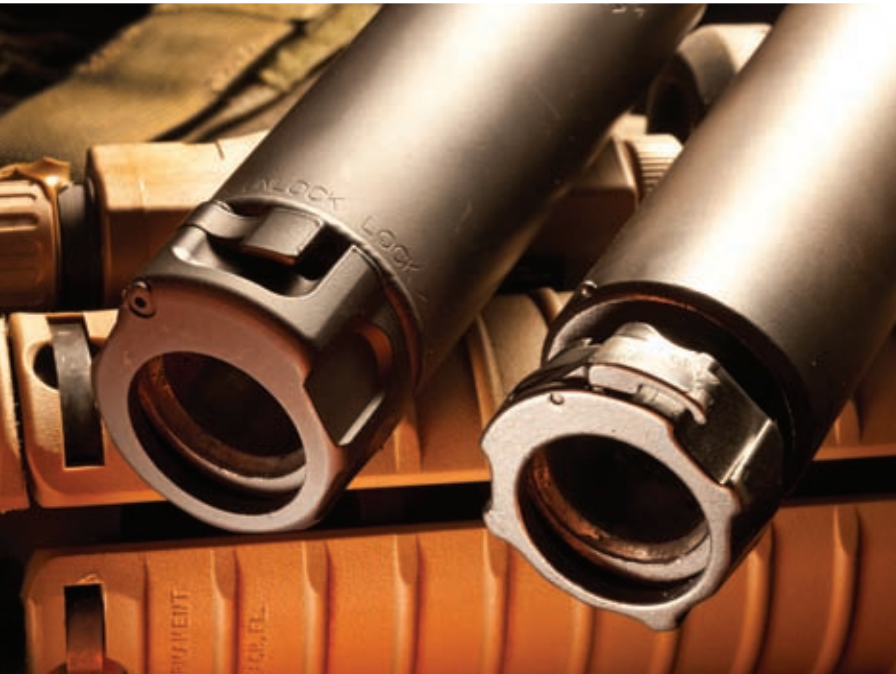
The previous generation locking ring (right) cinches itself to the adapter on the gun, while the "new and improved" version (which it really is) self-locks. Note again the recessed locking lever (left) compared to the more exposed lever on the earlier version.
